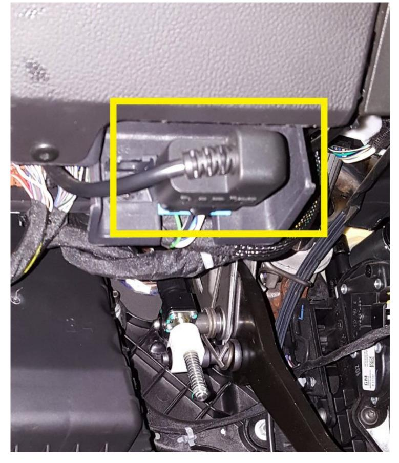
**2.** Remove the side dash cover using a plastic pry tool or screwdriver. Route the Starter Cable and OBD-II Cable to the iDash.
