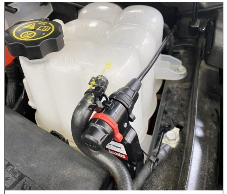
4. Locate a place to secure the Derringer module near or along the fender, then ziptie it in place. Ensure the LED indicator is viewable. If there is extra cable length, secure it out of the way with zip-ties.
